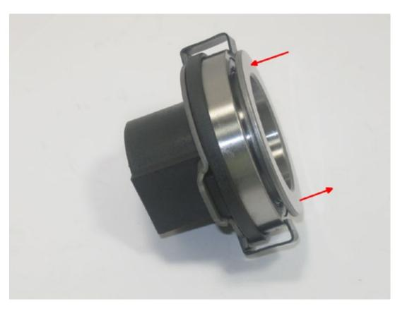
This is a design characteristic of the bearing and is not a defect
